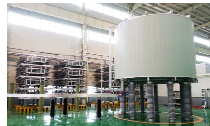
DC Temperature Rise Test on 800kV SMR at 6250A
