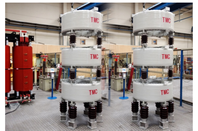
TMC Project in Spain 1850A Current Limiting Reactor
