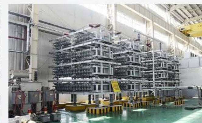
Capacitor Banks (up to 60kV) for AC Temperature Rise Testing
